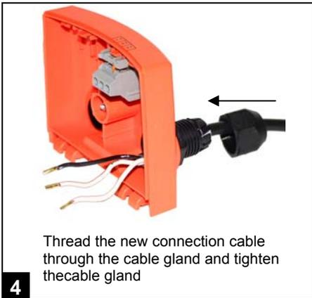
Thread the new connection cable through the cable gland and tighten the cable gland
